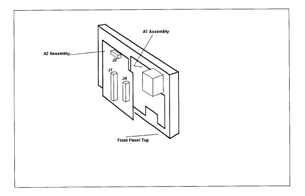
Figure 2 Location of Front Panel Board Assemblies
